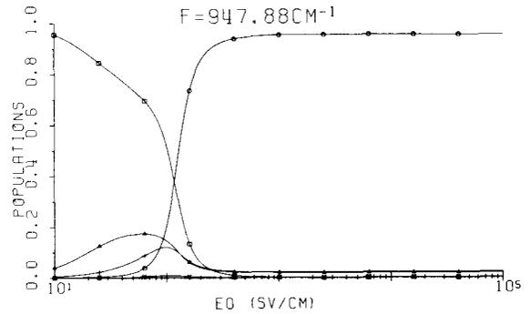
Fig. 2. Populations in the sublevels  $|1j\rangle$  of a  $(1, 5)$  system for which the upper-level spacing is  $\delta/2\pi c = 0.1 \text{ cm}^{-1}$ ; the transition dipole moments are  $\sum \mu_i^2 = (4 \times 10^{-19} \text{ st C} - \text{cm (esu)})^2$   $\square$ :  $|0, 0\rangle$  state;  $\circ$ :  $|1, 1\rangle$  state.
