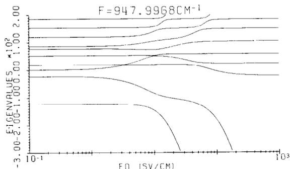
Fig. 3. Dressed-state eigenvalues  $\lambda$  of a (1, 3, 6) system as functions of the laser field amplitude  $E_0$ , showing avoided crossings. Parameters were (see fig. 1)  $\bar{\nu}_{10} = 948.000 \text{ cm}^{-1}$ ;  $\bar{\nu}_{21} = 947.985 \text{ cm}^{-1}$ ;  $\delta_1 = 0.01 \text{ cm}^{-1}$ ;  $\delta_2 = 0.0033 \text{ cm}^{-1}$ ;  $\Sigma \mu_i^2 = (4 \times 10^{-19} \text{ esu})^2$ ; and  $\omega/2\pi c = 947.98 \text{ cm}^{-1}$ .
