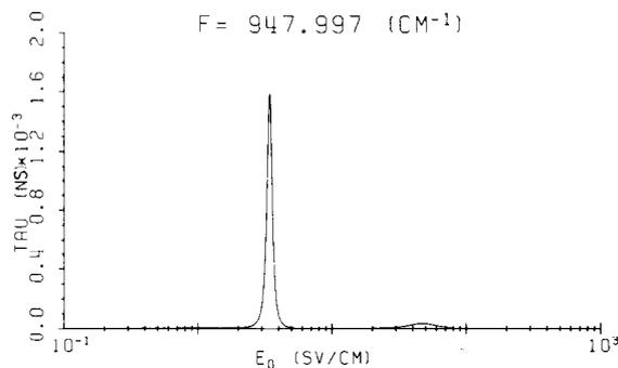
Fig. 5. The quantity  $T_p \equiv |\langle \lambda_0 | \Delta | \lambda_i \rangle| \omega_{i0}^{-2}$  as a function of laser field amplitude  $E_0$  for the (1, 3, 6) system of figs. 3 and 4. By (5a), the adiabatic approximation is obeyed for pulses that are long compared to  $T_p$ .
